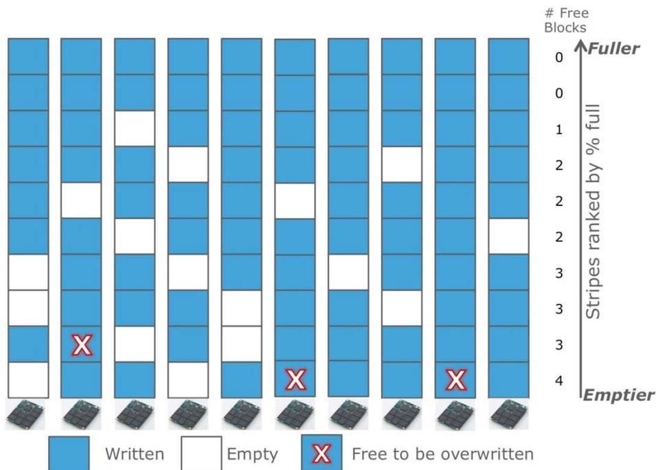
Figure 8. XDP ranks all stripes based on how full or empty they are and always writes to the emptiest stripe. In this simplified view there are ten data drives (columns) and ten stripes (rows). The emptiest stripes are ranked at the bottom. The example shows an array that is 80% full.
