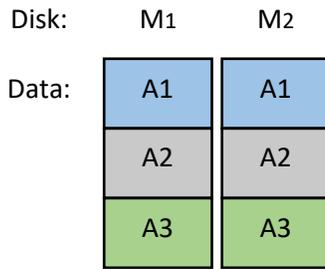
Figure 1. RAID 1 - All incoming writes are mirrored to two separate disks. This scheme has good rebuild performance, yet requires 50% capacity overhead. In the diagram, two disks are mirroring three blocks of data
