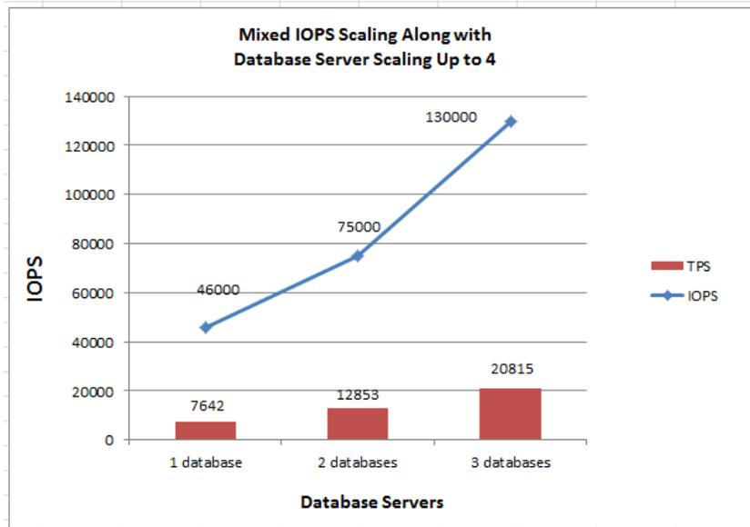
Figure 4. IOPS and TPS scalability of mixed workload
