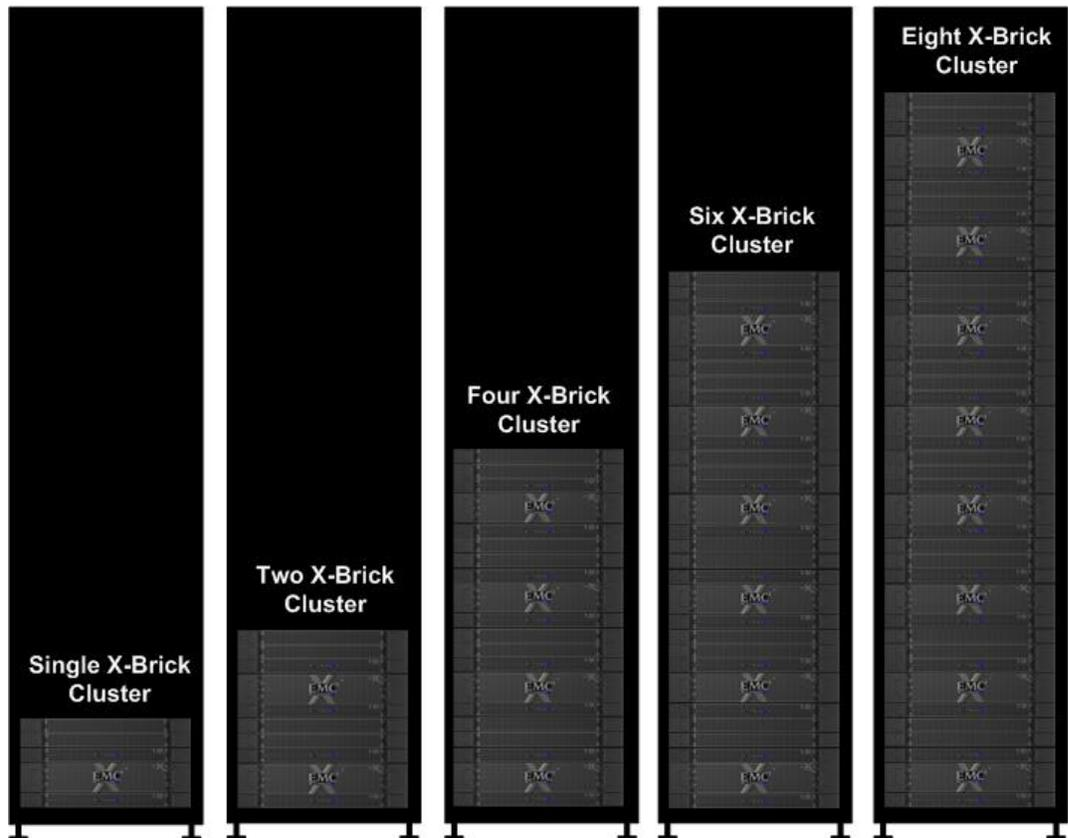
Figure 1. EMC XtremIO configuration for multiple X-Brick clusters
