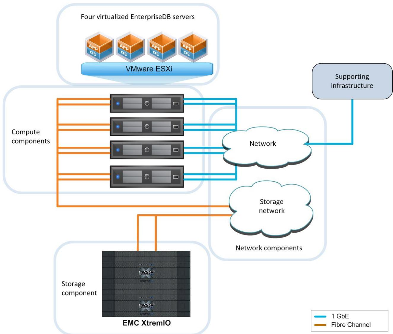
**Figure 2. Solution reference architecture**
