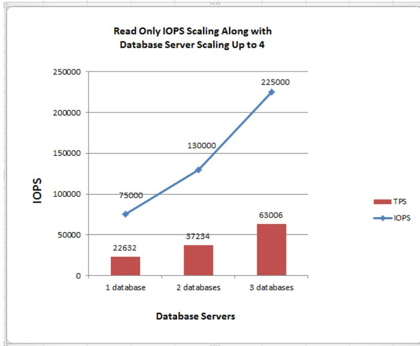
**Figure 3. IOPS and TPS scalability of read-only workload**
