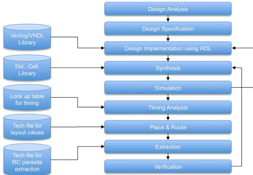
**Figure 1. A simplified digital design flow for EDA.**
