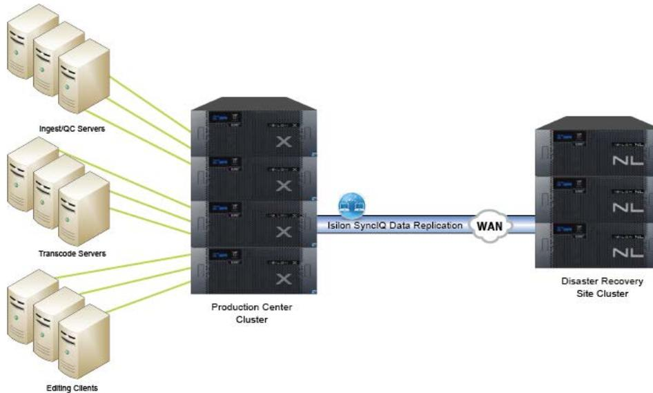
Figure 4. A MAM infrastructure based on Isilon scale out storage benefits from raw disk utilization rates up to 80% and eliminates network bandwidth associated with files copies between silos of storage.
