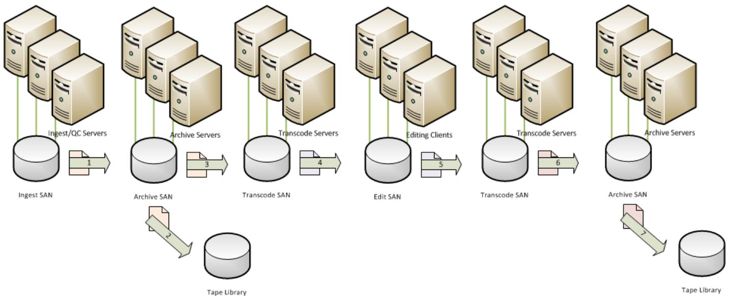
Figure 3. Typical SAN-centric MAM workflow requiring file movement between multiple silos of storage. LUN-based SAN storage architectures can typically achieve 50% or less storage utilization efficiency.
