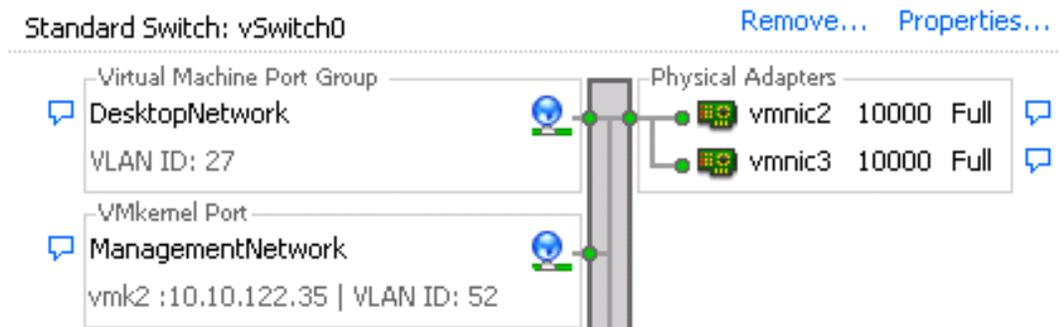
**Figure 4.** vSwitch configuration in the VMware vCenter server
