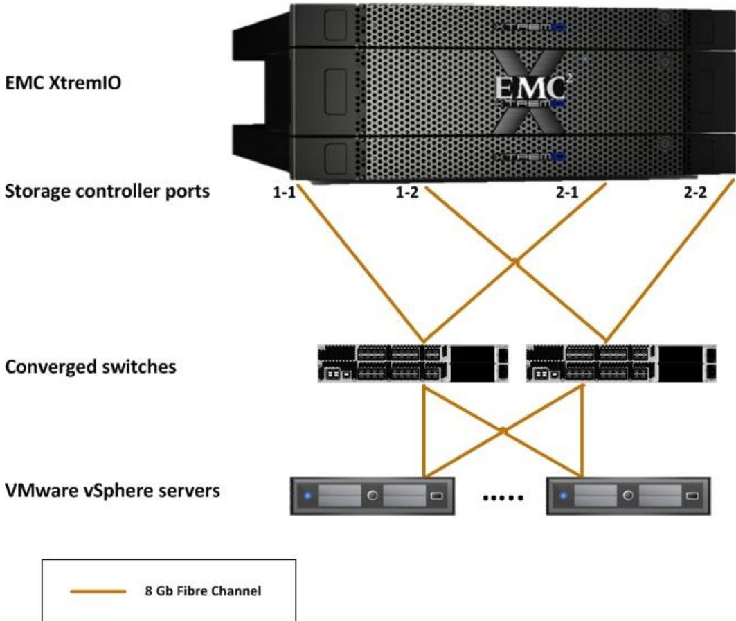
**Figure 3. Network layout diagram**
