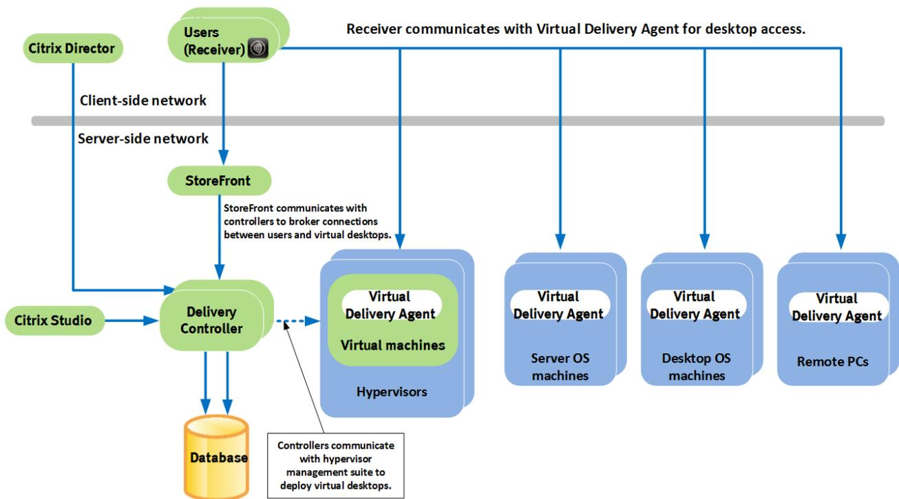
**Figure 3. XenDesktop 7.1 architecture components**
