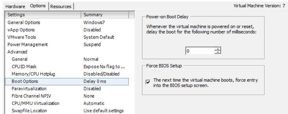
**Figure 3** Forcing the virtual machine into BIOS
