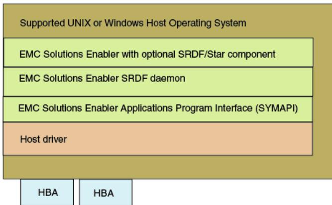
Figure 3. Host components for SRDF/Star
