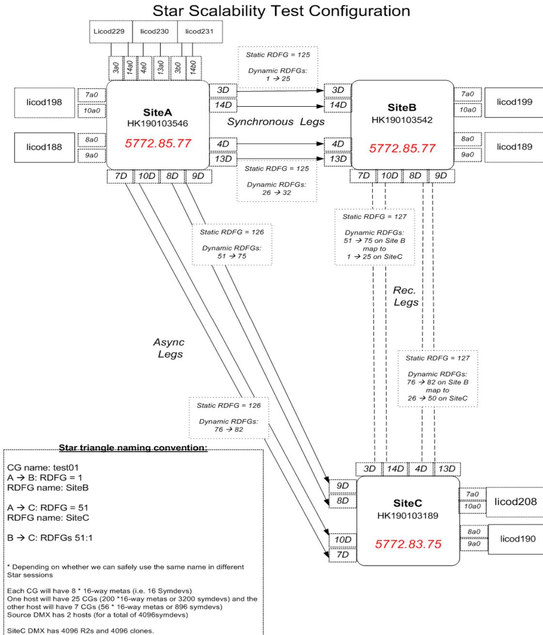
Figure 6. A detailed SRDF/Star design diagram
