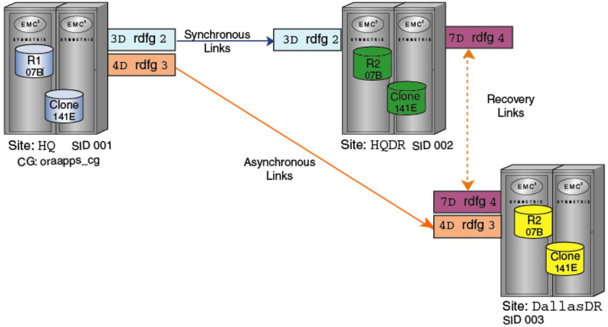
Figure 5. Basic SRDF/Star component design
