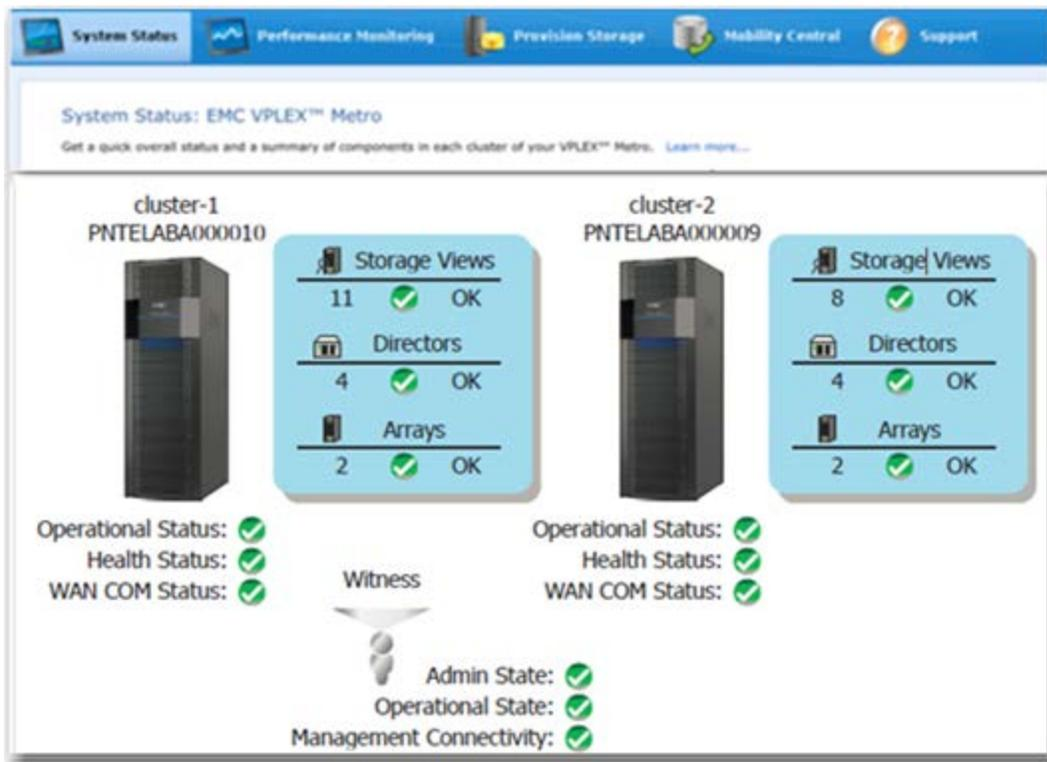
Figure 7. EMC Unisphere for VPLEX management interface
