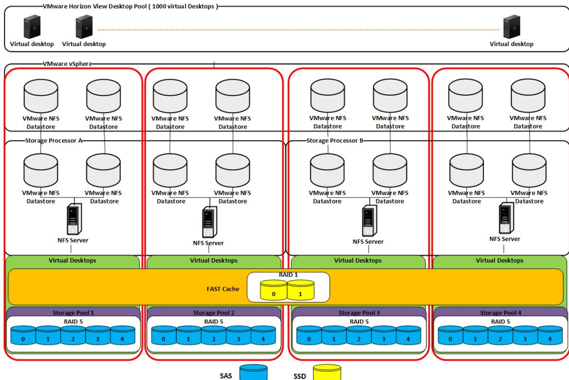
**Figure 3. Storage building block for desktops**
