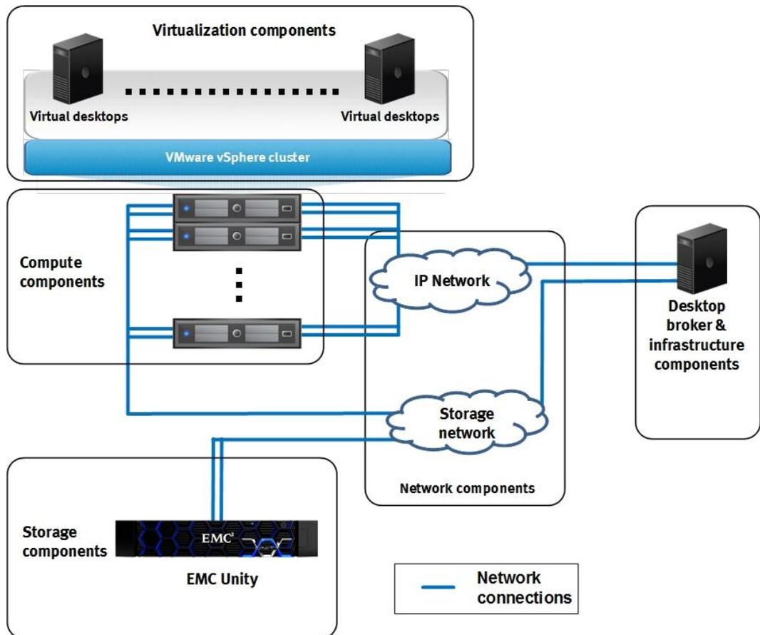
**Figure 1. Architecture of the validated solution**
