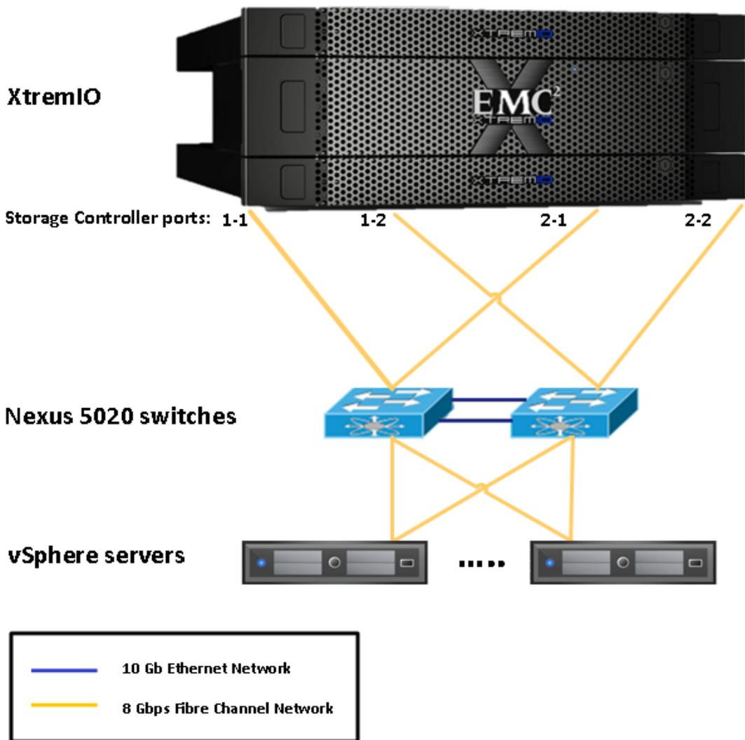
Figure 2. Network layout diagram
