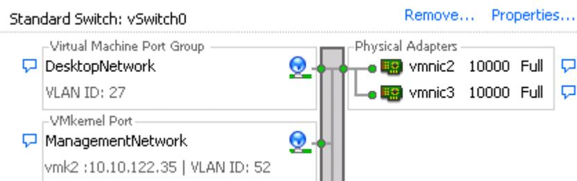
Figure 3. vSwitch configuration in vCenter Server
