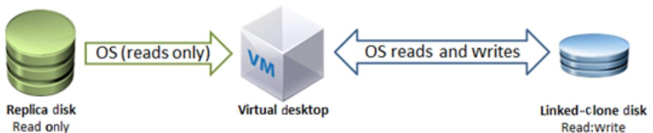
**Figure 4. Logical representation of replica disk and linked clone**
