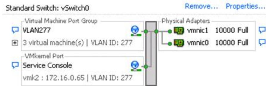
**Figure 4.** vSwitch configuration in vCenter Server
