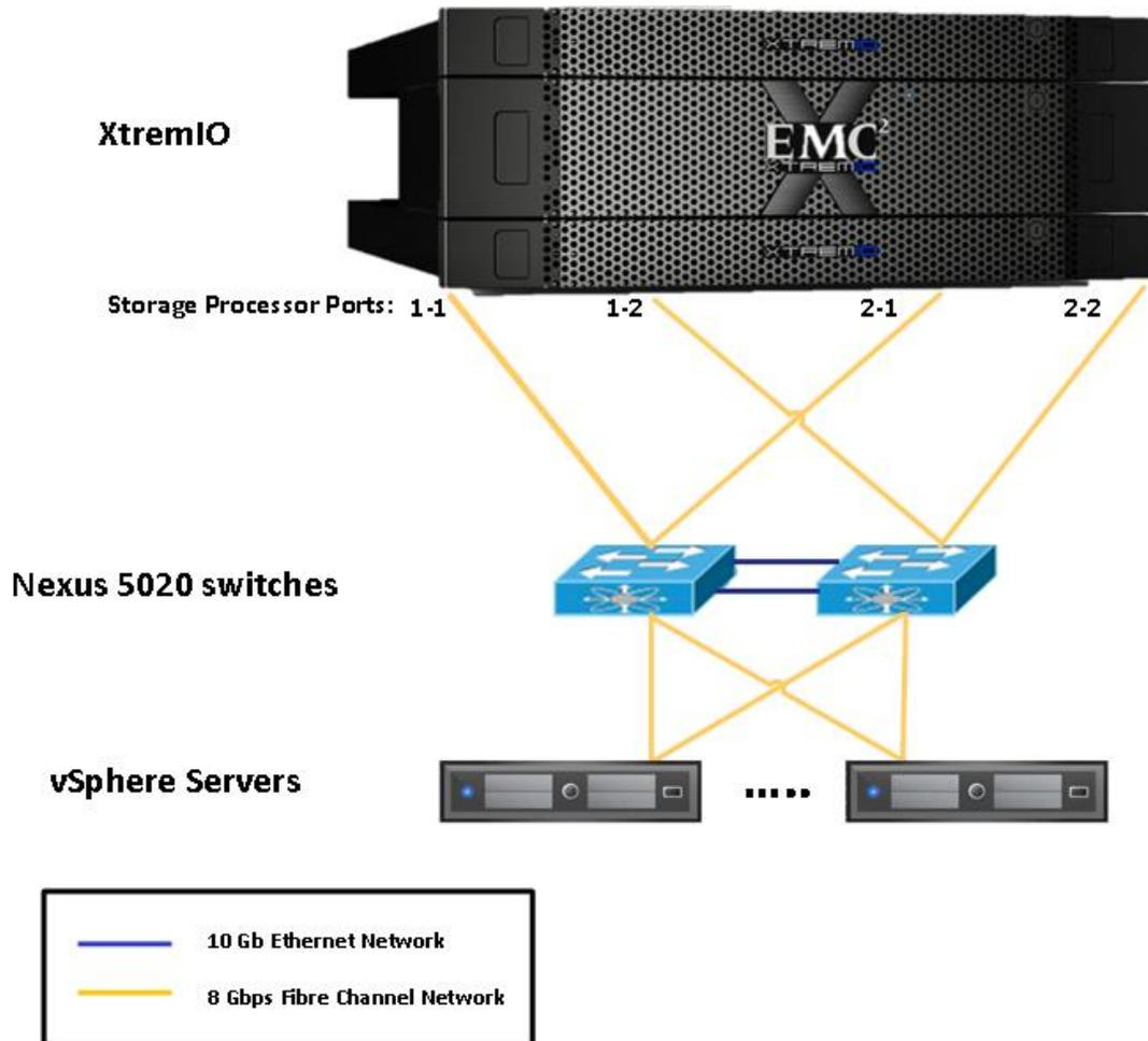
Figure 2. Network layout diagram
