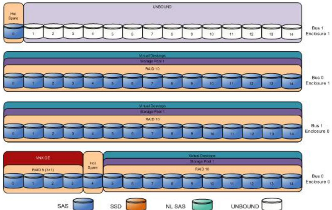
**Figure 2. Core storage layout**
