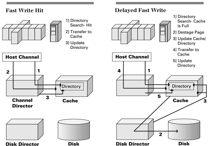
A *Fast Write* occurs when the percentage of modified data in cache is less than the Fast Write threshold. On a host write command, the Channel Director places the incoming block(s) in cache.
