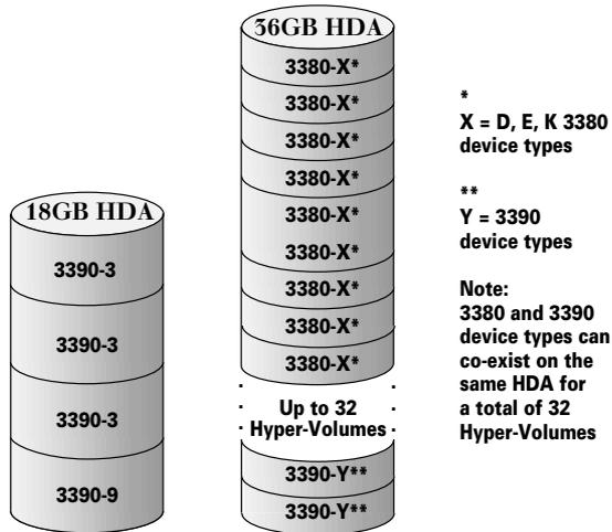
Open systems customers can also take advantage of Hyper-Volume Extension to support multiple logical disk volumes on individual disks. This capability is particularly useful for some 32-bit implementations of UNIX that allow only 2GB file systems per single logical disk. For example, up to eight 2GB logical disk volumes can be defined for a single EMC 18GB HDA.
