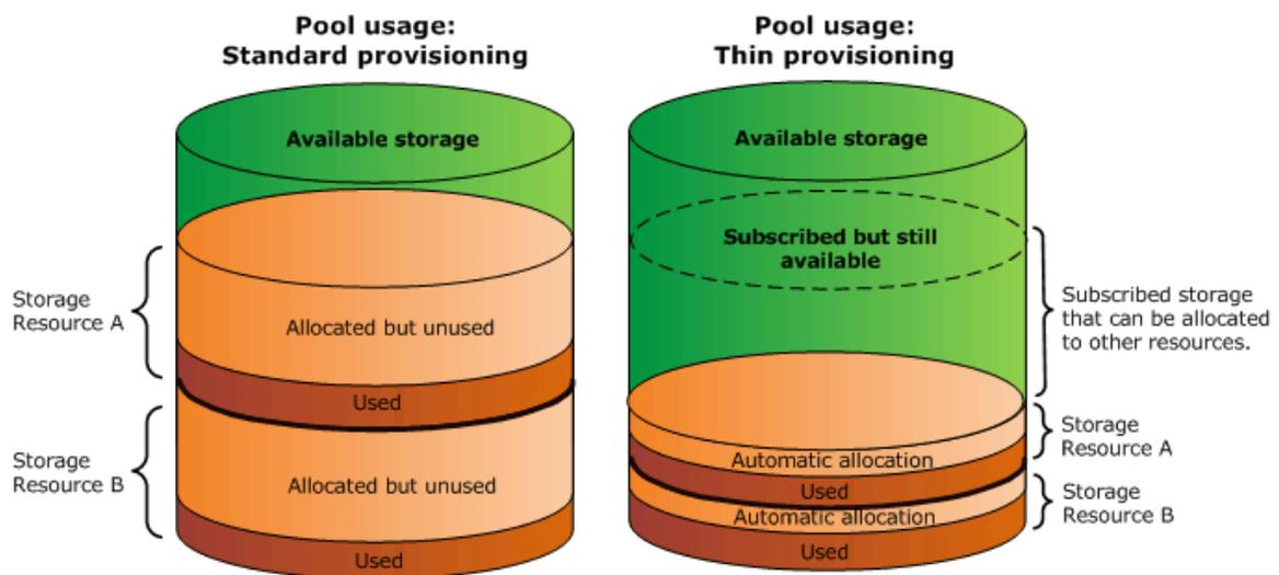
Figure 8. Comparison between standard provisioning and thin provisioning
