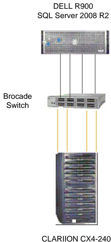
**Figure 1. CLARiiON CX4 hardware configuration**
