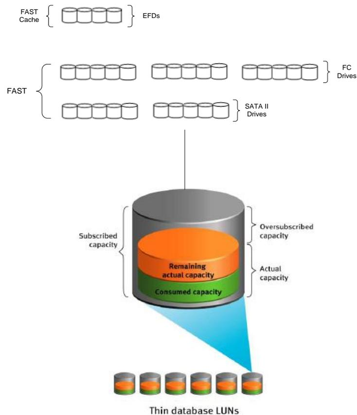
**Figure 3. Storage layout for the use case**
