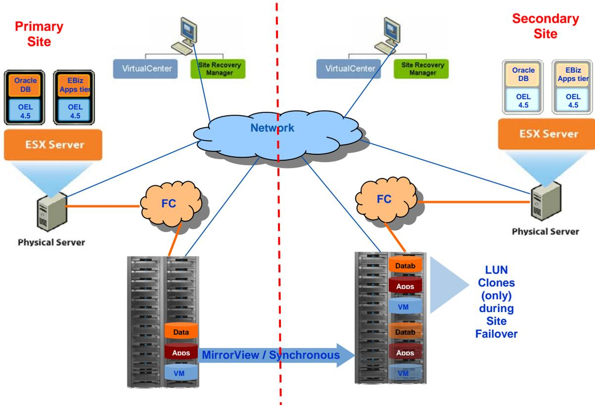
Figure 5. Site Recovery Manager configuration with CLARiiON CX4-480 storage
