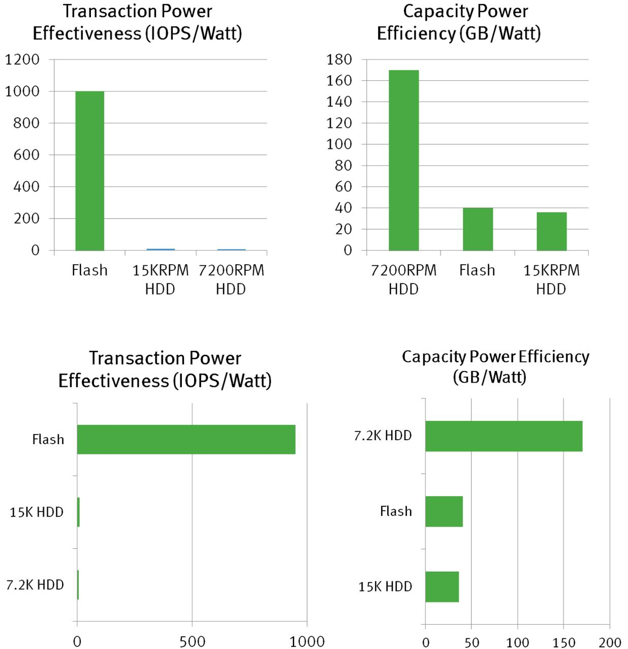
Figure 1 Drive Efficiency
