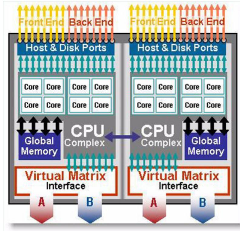
Figure 1 Symmetrix V-Max high availability node layout
