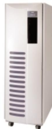
*The Symmetrix 8530 is a single-bay, high-performance, networked storage system with up to 64GB of cache; up to 17.2TB of capacity; support for Fibre Channel (up to 72 ports); Ultra/Ultra 2 SCSI (up to 24 ports); ESCON (up to 24 ports); FICON (up to 16 ports); or a combination of all connectivity types.*
