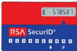
The RSA SecurID 520 PINpad model is the same size as the RSA SecurID 200 but has a PINpad feature that enables users to encrypt their passcode for a higher level of security.
