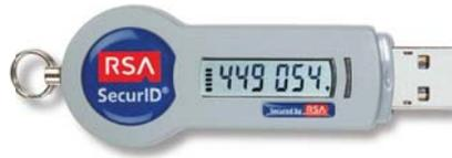
The RSA SecurID 800 offers the one-time password functionality of the other hardware authenticators and can be used for storage of Windows® username/password credentials and digital certificates—creating a master key for multiple authentication methods. When connected, the RSA SecurID 800 is enabled for automatic token code entry, allowing applications to programmatically access token codes directly off the device and eliminating the need for the user to type their code.
