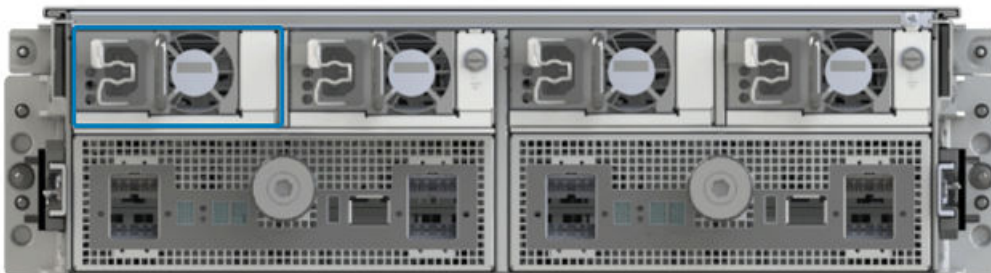
Figure 7 Replacement power/supply B0 - example location
