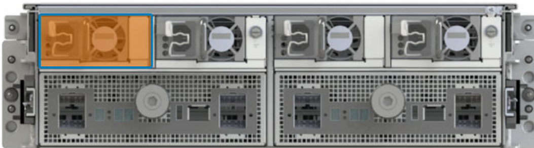
Figure 1 Faulted power supply B0 - example location
