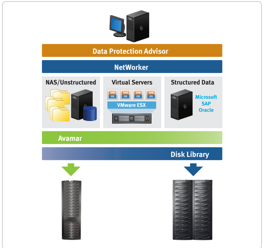
Figure 2: Data Protection Advisor for the entire backup infrastructure further increases Avamar management efficiency by integrating backup application, disk library information, and more for increased visibility and insight.
