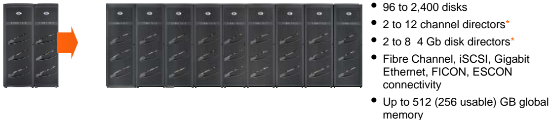
Figure 2. Symmetrix DMX-4: World's largest high-end storage array
