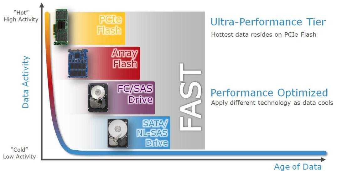
**Figure 5.** XtremCache and FAST automatically tier hot and cold data
