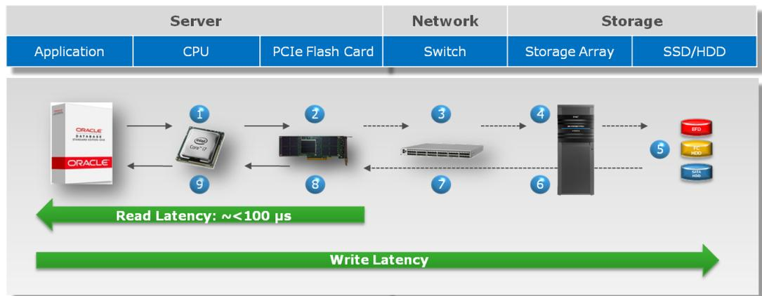
**Figure 4. Advanced architecture with EMC XtremCache**
